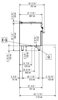
EQ = Equipotential screwG = Gas connection
